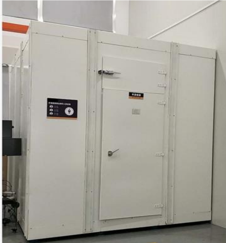
Noise Testing Anechoic Chamber
